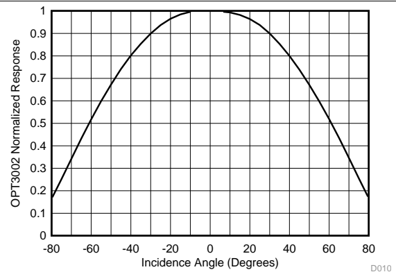
Figure 9. Normalized Response vs Incidence Angle
